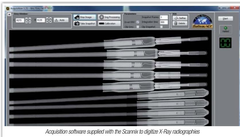
Acquisition software supplied with the Scannix to digitize X-Ray radiographies
