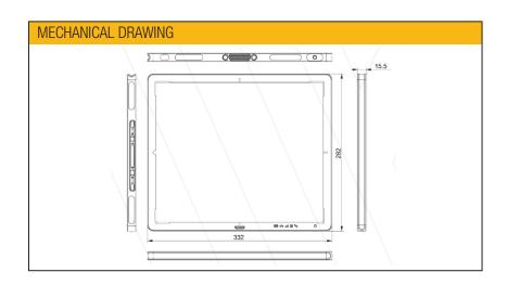
The MOBIX 16-100 is a portable flat panel detector. Thanks to its battery and Wi-Fi interface, a digital inspection can now be done anywhere. Moreover the MOBIX 16-100 is very light, robust and ergonomic which makes it easy to be used in harsh environment and conditions. Equipped with an internal memory, the MOBIX 16-100 can store images in order to allow the operator to unload them later.
